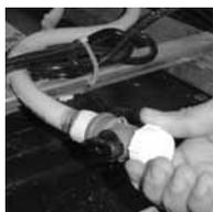
1. **DRAINING YOUR RIVIERA SPA.** The drain is located behind the front panel on the far right side, grasp the hose bib cap and turn it counter clockwise. Attach a garden hose, if desired. Turn the black knob on the side of the valve a quarter turn. Draining times may vary by model using the external hose bib. A sump pump may also be used to drain the spa quickly.
